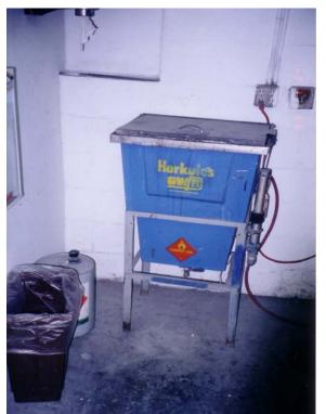
Figure 2-2. Spray Gun Cleaning Unit at Autobody Shop #2
