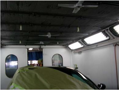
Figure 3-15. Coating Booth with Three Ceiling Fans
