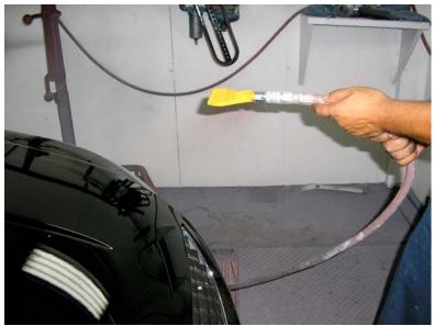
Figure 3-17. Painter Using Drying Tool
