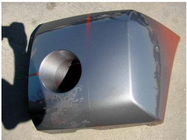
Figure 2-5. Scrap Part with Four Coating/Thinner Combinations at Autobody Shop #4
