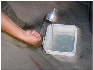
Figure 2-12. Bucket For Cleaning Spray Gun With Tap Water at Autobody Shop #6
