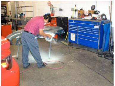
Figure 4-1. Sanding with Six Hole Sanding Disc
