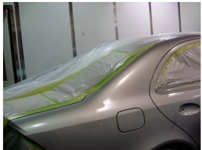
Figure 3-12. Car Painted With Waterborne Base Coat at Autobody Shop #6
