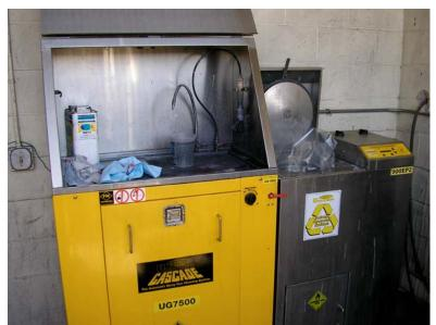
Figure 2-3. Spray Gun Cleaning Unit at Autobody Shop #4
