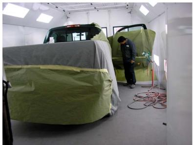
Figure 3-10. Painter Inspecting Truck Painted with Waterborne Base Coat at Autobody Shop #6
