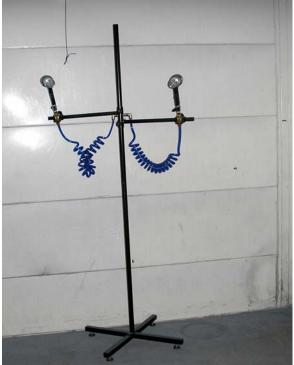
Figure 3-6. Portable Drying System at Autobody Shop#4
