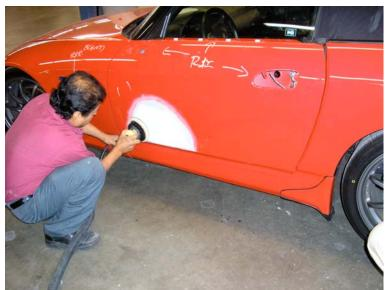
Figure 4-2. Sanding with Mirka Sanding Disc
