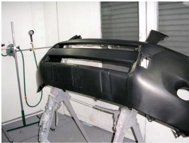
Figure 3-16. Coating Booth with Portable Dryers
